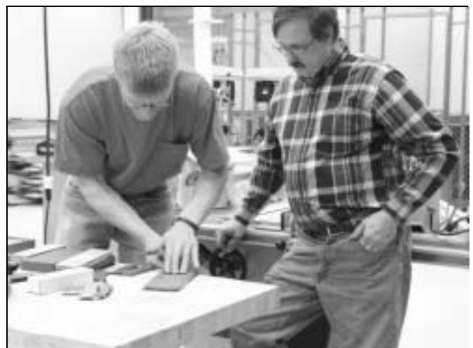
John Kirchoff demonstrates flattening the back of an iron.
