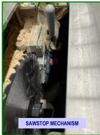
ED & GREG— EXAMING THE BRAKE AND BLADE ASSEMBLY
