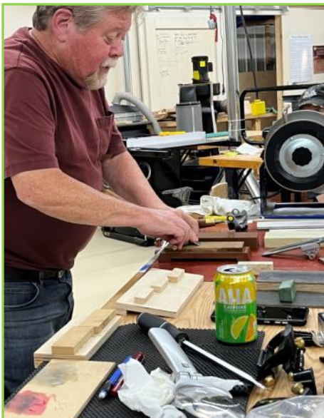
Don Peterson discussed tool sharpening with waterstones and diamond plates using tool holders and guides.
