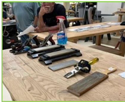
L to R: 3 wood planes, 2 Japanese sharpening stones w/ holding frames, a diamond lap plate, chisel and chisel holder for sharpening, and a leather strop for a final honing.
