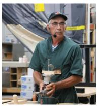
A small fence attached directly to the router base
