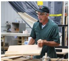
Sled for use on the router table. Allows you to safely hold and cut parts of different sizes.
