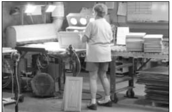
Final inspections happen under many lights and any imperfections are fixed.
