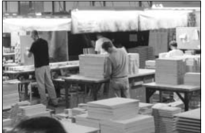
Woodcraft employees assemble raised panel doors using glue with a dye that fluoresces in ultra-violet illumination.
