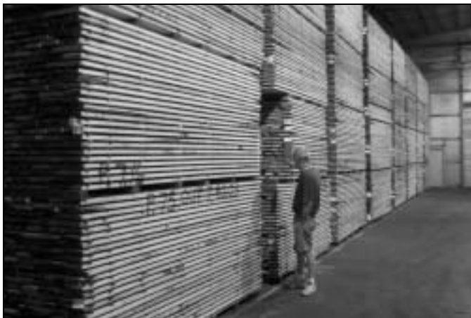
The St. Cloud Facility can dry hundreds of thousands of board feet of green lumber in their kilns. Scrap lumber from the plant is burned in a furnace to heat the kilns.
