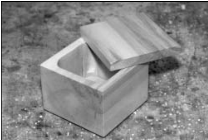
Ron McKeever made this band saw box from a solid chunk of oak.
