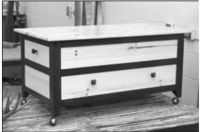
John Caye made this functional coffee table from yellow poplar. He used mortis and tenon construction.
