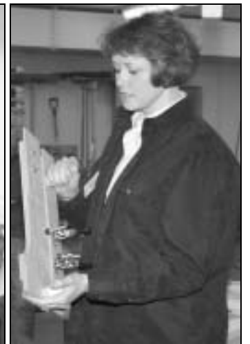
David Schwanke (left) uses belt sander sandpaper around a wooden block to quickly remove material. Cindy Johnson made this jig to cut the legs on her boxes.
