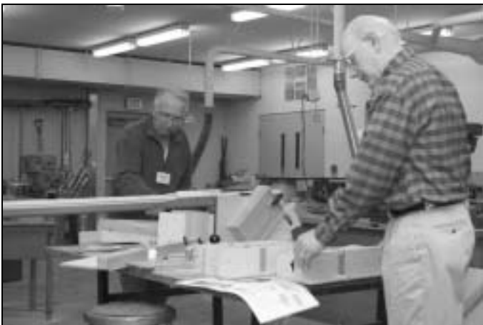
Alex Neussendorfer (right) built this finger joint jig from a plan in Shop Notes magazine. The jig allowed cutting finger joints quickly and accurately as well as allowing for many sized fingers.
