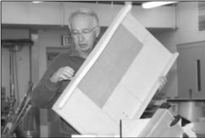
John Caye demonstrates his crosscut sled for the table saw. John has glued sandpaper to the top surface to keep the work piece in place and laminated the bottom for low friction use.
