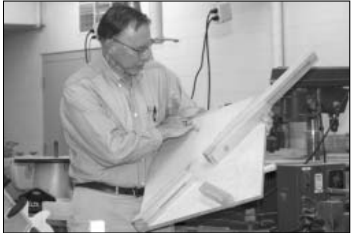
Byron John uses this miter sled on his table saw to cut perfect miters.
