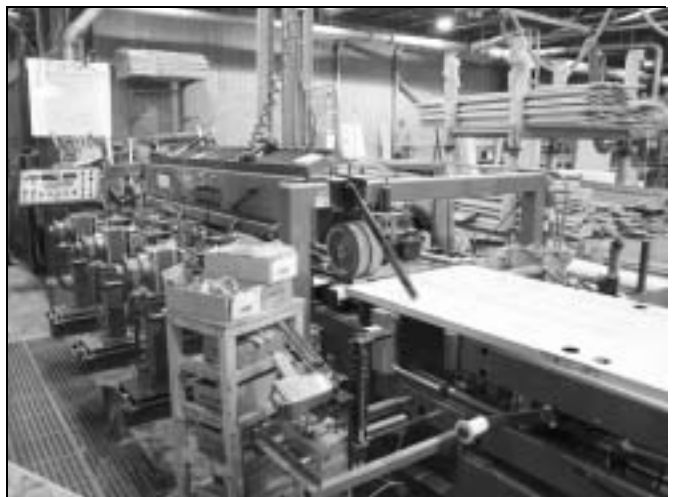
Pre-hung doors are mechanically assembled using the Norfield 5000.
