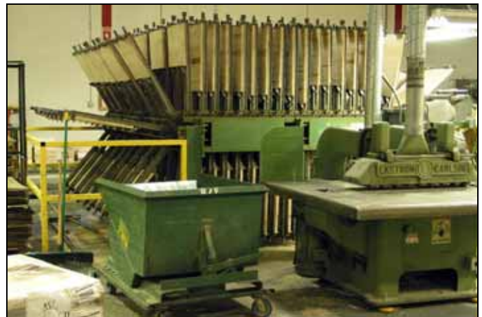
Woodcraft has many specialized machines like this clamping station.
