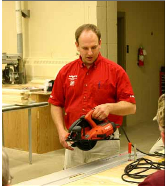
Demonstrating Hilti's WGS 1400-2 Guide Rail, Greg showed how the guide makes quick work of sheets of plywood.
