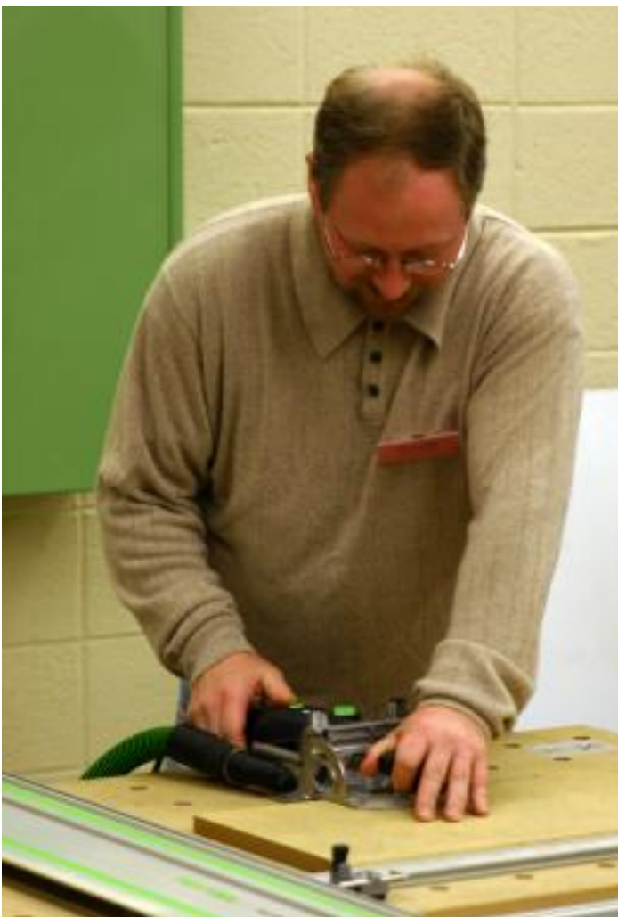
The DF 500 Domino Joiner makes mortise for pre-fabricated tenons. Scott Randall gives it a spin.
