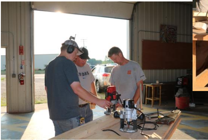
Cutting the bench tops to length and routing the top to mount the two face vices.
