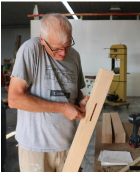
Legs are mortised and drilled for joining to the stretchers
