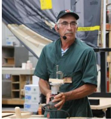
A small fence attached directly to the router base
