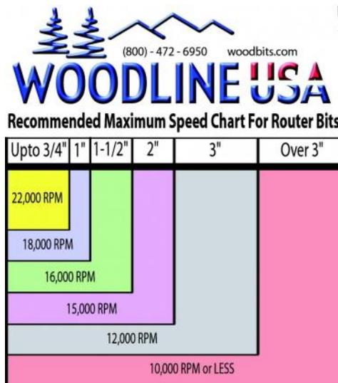
In order to maintain a safe woodworking environment it is necessary to adjust the speed of your router to accommodate the size and design of the router bit. This speed chart has been designed as a quick reference of recommended speeds based on bit diameter. Remember these are a recommendation only and some bit types or profiles may require slower speeds. Slower operation will often produce a cleaner cut with less burning and tear out while extending the life of the bit.
